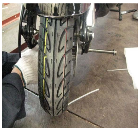
15: Insert spacer, put front wheel & speed sensor in place.
