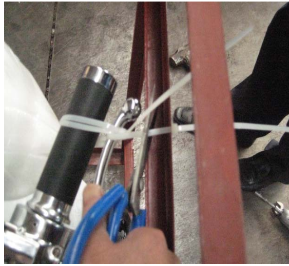
5: Cut wire ties from handle bars.
