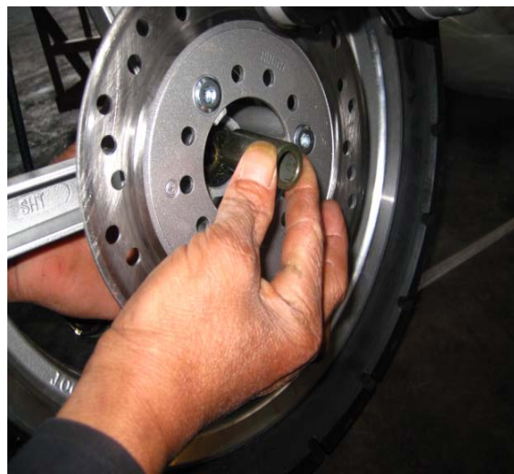
15: Insert spacer, put front wheel & speed sensor in place.
