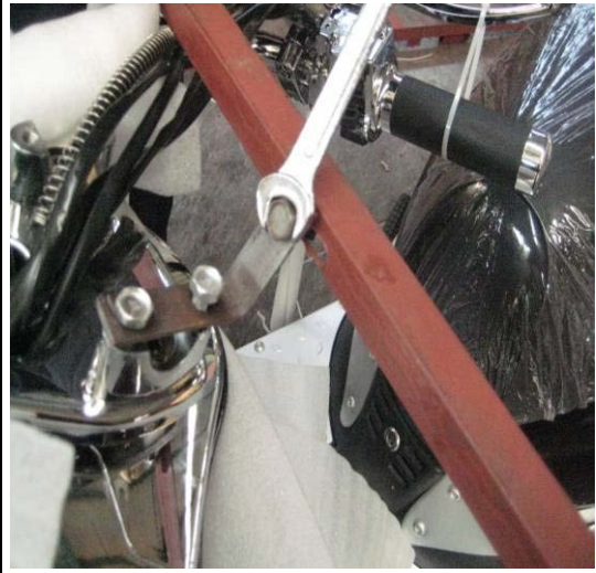
6: Remove bolts for front fork.
