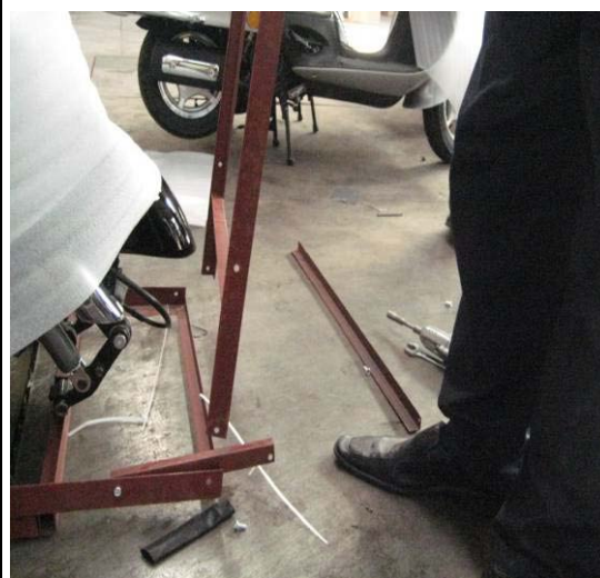
8: Pull upper frame up carefully.
